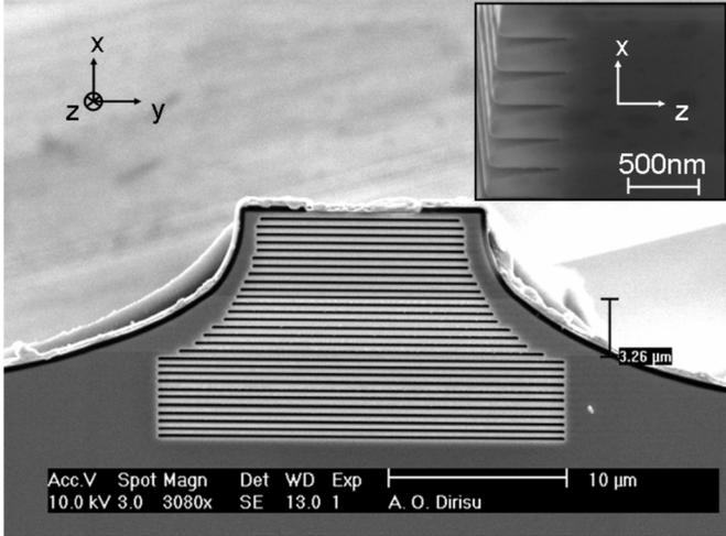
Fig. 1. Scanning electron microscope (SEM) image of a QCL facet milled with horizontal gratings. The inset shows a cross section of the gratings along the length of the laser ridge (the  $z$  direction).
