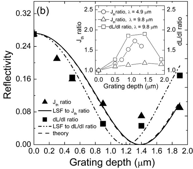
Fig. 3. Reflectivity versus the grating depth for  $\lambda = 9.8 \mu\text{m}$  using  $J_{\text{th}}$  ratio and  $dL/dI$  ratio. LSF indicates the least squares fit to the data with  $n_f$  as the fit parameter in (2). The inset shows the experimental data of the threshold current ratio and slope efficiency ratio for different depths; the connecting lines serve as guides for the eyes.
