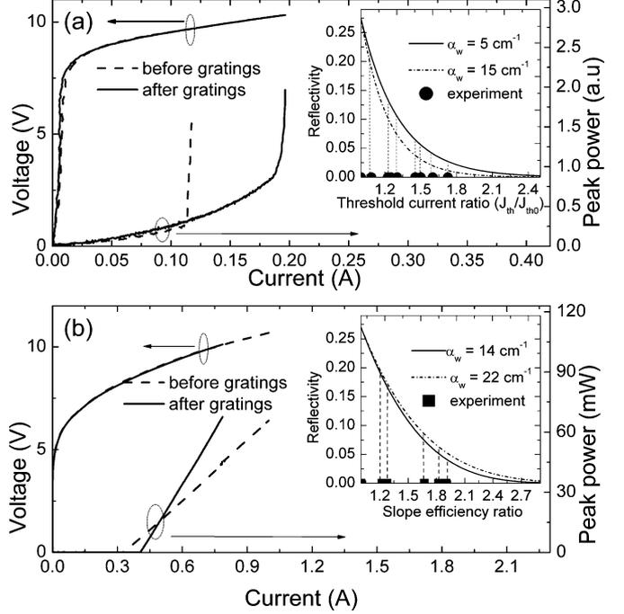
Fig. 2.  $L-I-V$  measurements showing the threshold shift and change in slope efficiency before and after milling the gratings. (a)  $\lambda = 4.9 \mu m$ . The inset shows the reflectivity versus threshold current ratio,  $L_{cav} = 0.05$  cm for  $\alpha_w = 5$  and  $15$   $cm^{-1}$ . (b)  $\lambda = 9.8 \mu m$ . The inset shows the reflectivity versus slope efficiency ratio,  $L_{cav} = 0.15$  cm for  $\alpha_w = 14$  and  $22$   $cm^{-1}$ .
