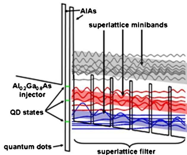
FIG. 1. (Color online) Conduction-band structure for a multiple wavelength mid-IR emitter at 20 kV/cm bias. The quantum dot layer is depicted schematically as a narrow quantum well. States in the superlattice are shown by their modulus squared, and the extraction minibands are shaded to aid in viewing.
