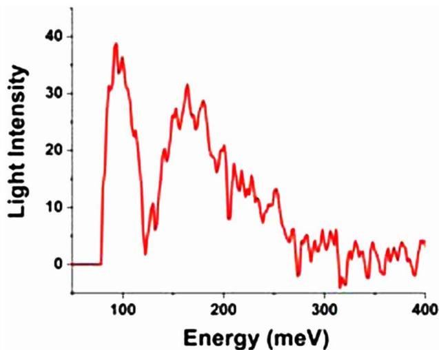
FIG. 2. (Color online) Electroluminescence spectrum for a multiple wavelength mid-IR QD emitter. The sample was operated in pulsed mode (20 kHz, 20  $\mu$ s pulse width) at a voltage corresponding to an electric field of 20 kV/cm across the active region. Two distinct emission peaks can be seen at about 100 and 175 meV.
