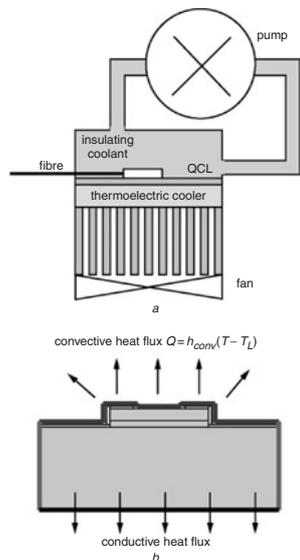
**Fig. 1** Schematic of QC laser (QCL) packaging module for direct liquid cooling, and schematic of heat transfer mechanisms involved in direct liquid cooling packaging
