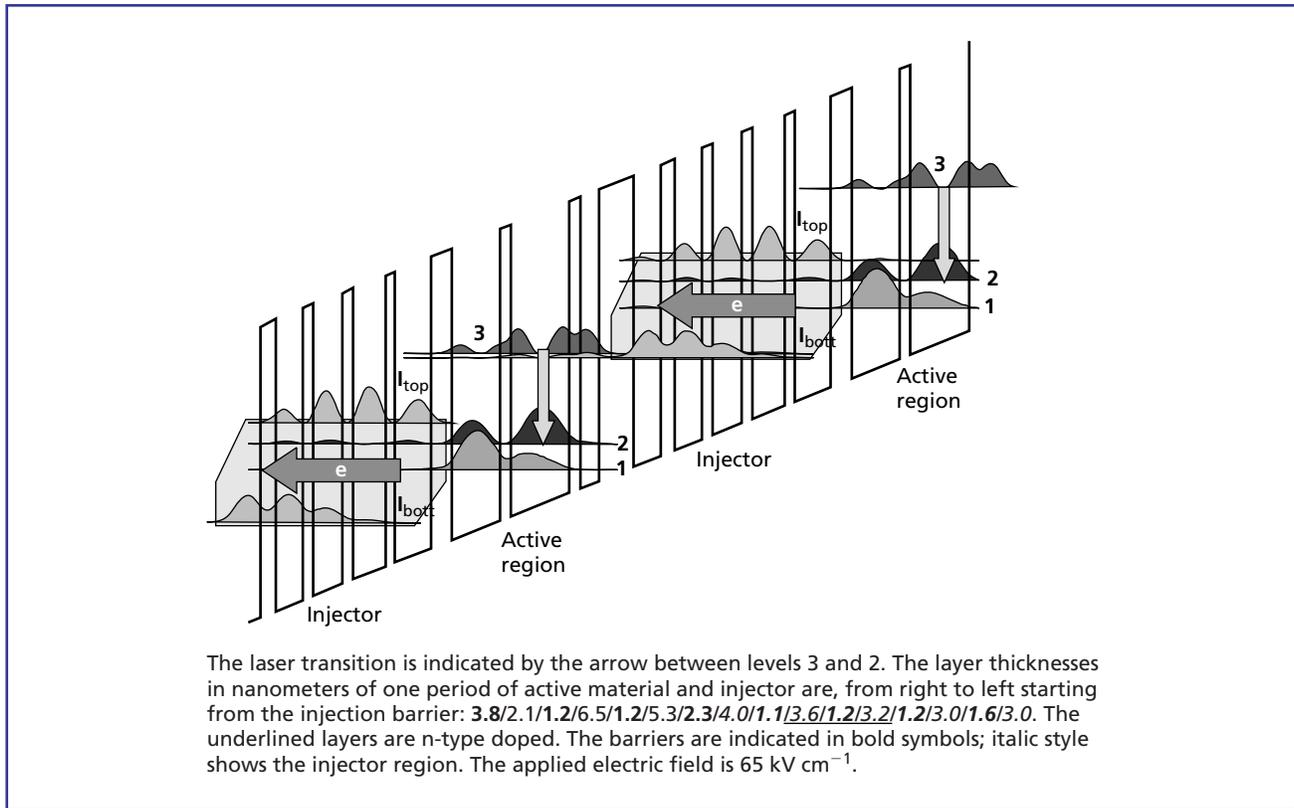
**Figure 2.** Conduction band diagram of the active and injector regions of an 8 μm QCL and the moduli squared of the most significant wavefunctions.
