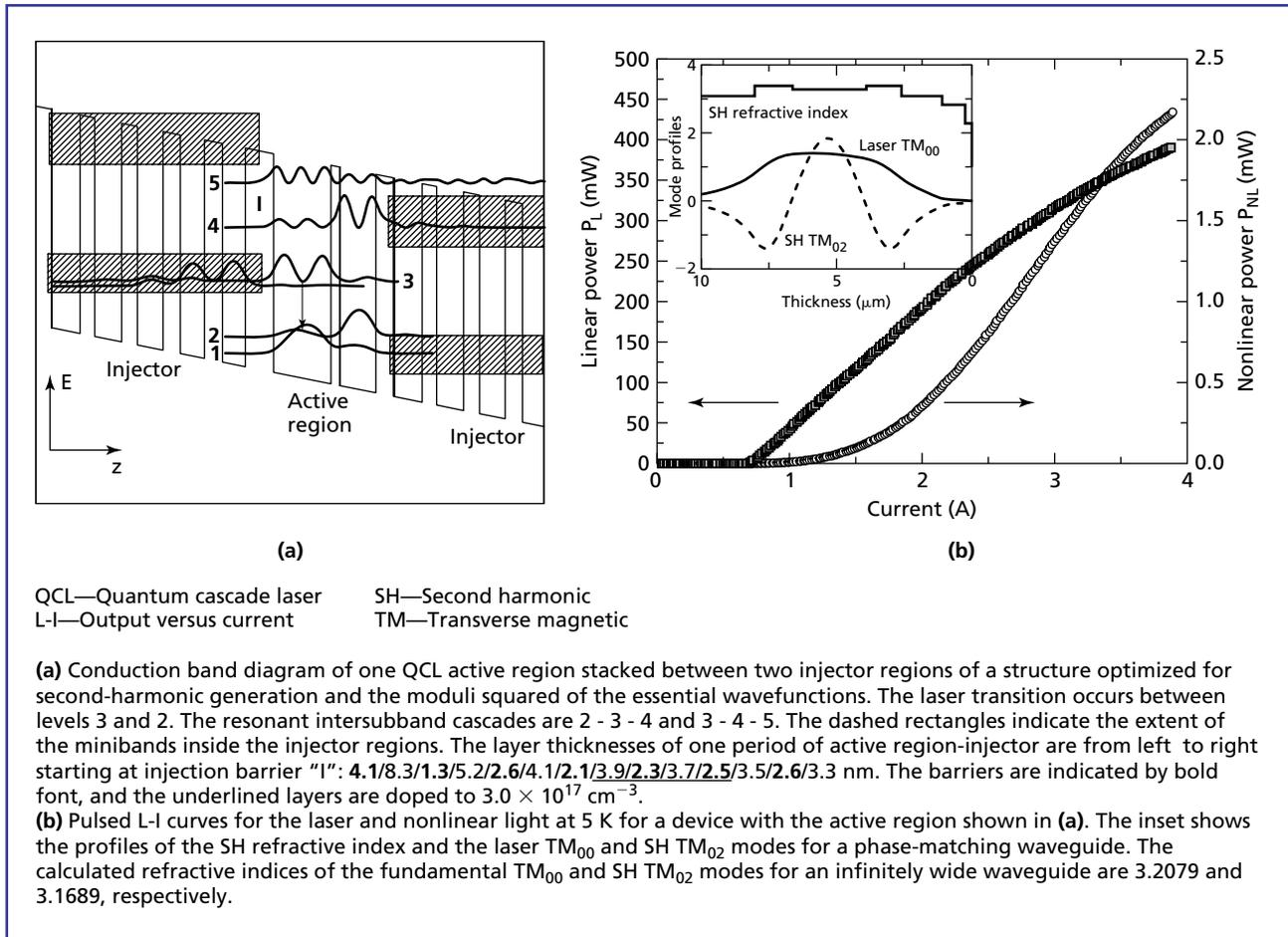
**Figure 5.** Structure and performance of a nonlinear QCL emitting fundamental light at  $9 \mu\text{m}$  and second-harmonic light at  $4.5 \mu\text{m}$ .
