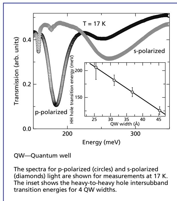
**Figure 6.** Mid-infrared intersubband transmission spectra of a sample containing 31  $\text{\AA}$  wide, carbon modulation-doped GaAs QWs with digital  $\text{Al}_{0.57}\text{Ga}_{0.43}\text{As}$  alloy barriers.
