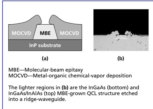
**Figure 7.** Schematics of the InP MOCVD overgrowth process (a) and side image of a deep-etched ridge-waveguide (b) on which InP (darker regions) was grown by MOCVD.
