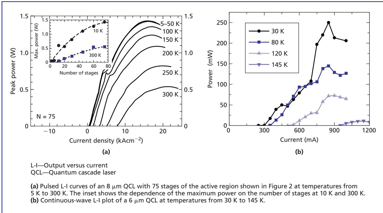
**Figure 4.** QCL performance characterization in pulsed and continuous-wave operation modes.
