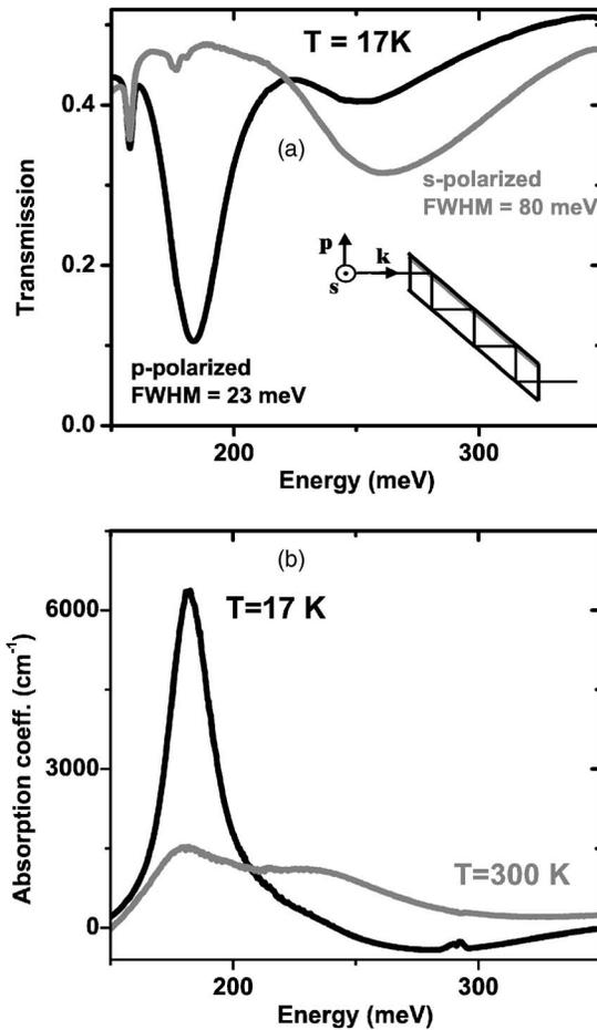
FIG. 1. (a) Midinfrared intersubband transmission spectra of the sample containing 31 Å wide carbon modulation-doped GaAs QWs with digital  $\text{Al}_{0.57}\text{Ga}_{0.43}\text{As}$  alloy barriers. The spectra for  $p$ -polarized (black line) and  $s$ -polarized (gray line) light are shown for measurements at 17 K. The inset shows the experimental multipass waveguide geometry. (b) Absorption coefficient for the 31 Å QW sample at 17 K (black line) and 300 K (gray line).
