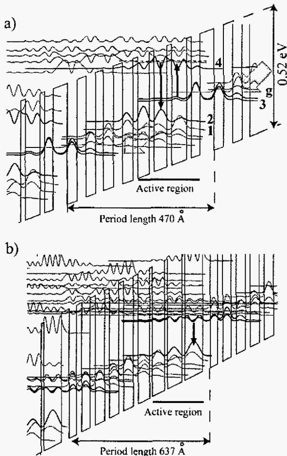
Fig. 1. Conduction band diagram of the (a) nonlinear and (b) pump regions in wafer D3015. The InGaAs wells and AlInAs barriers are grown lattice matched to InP substrate. The moduli squared of the relevant wave-functions are also shown. In (a), the black arrows indicate the Raman transition, while the grey arrows show the electron transport through the injector regions. In (b), the black arrow indicates the laser transition.
