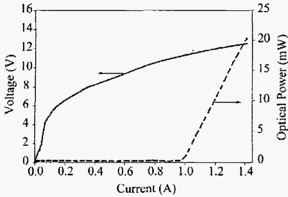
Fig. 4. Light output and voltage versus current characteristics of the laser corresponding to wafer D3015. This measurement was carried out at liquid nitrogen temperatures.
