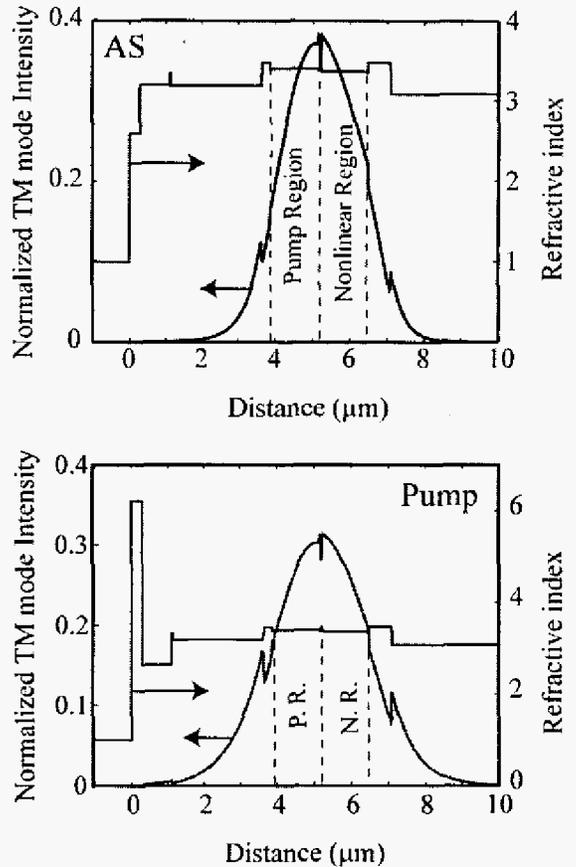
Fig. 2. Normalized intensity mode profile and profile of the real part of the refractive index in the (reverse) growth direction for both Anti-Stokes and pump fundamental modes in D3015.
