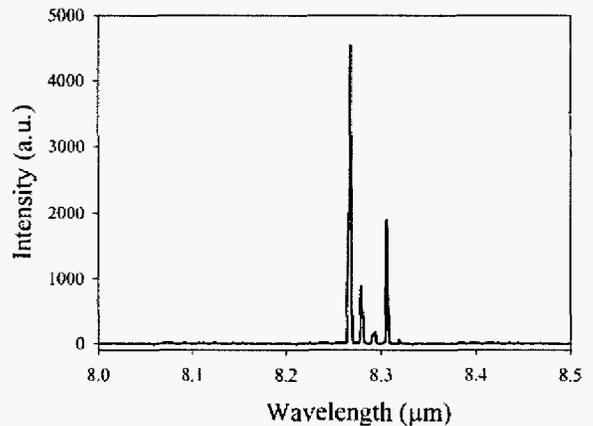
Fig. 3. Spectrum showing the pump laser emission in D3015 for 3A peak current. The measurements have been taken at cryogenic (liquid nitrogen) temperature and in pulsed current mode using a Nicolet 860 FTIR.
