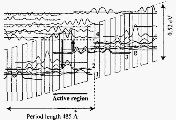
Fig. 6. Conduction band diagram of the nonlinear region in D2924. In a similar fashion to Fig. 1, the moduli squared of the relevant wave-functions are also plotted. The AS Raman transition is again indicated by black arrows.
