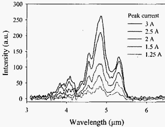
Fig. 5. Short wavelength emission spectra of D3015 above laser threshold. Peaks attributed to stimulated Anti-Stokes emission (4.8  $\mu\text{m}$ ) and incoherent upconversion (5.3  $\mu\text{m}$ ) can be distinguished. The dip observed around 4.3  $\mu\text{m}$  is characteristic of  $\text{CO}_2$  absorption.
