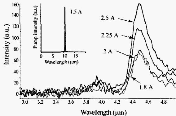
Fig. 7. Short wavelength luminescence spectra, above threshold, of D2924. The main peak at 4.5  $\mu\text{m}$  is attributed to stimulated Anti-Stokes emission. The inset shows the pump spectrum at  $\sim 90$  K for a peak current of 1.5 A.
