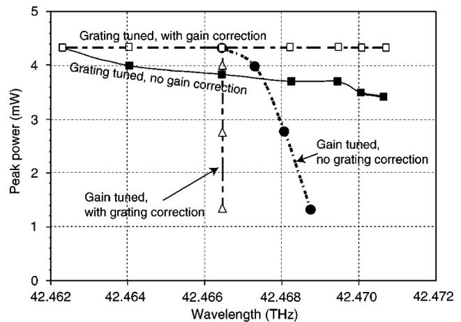
FIG. 4. External cavity laser power and wavelength control by combining gain and the Bragg grating (BG) segment currents. Filled squares: power variation as wavelength was tuned with BG segment alone. Open squares: Power corrected (maintained constant) with a gain current correction. Varying the power via the gain segment alone also resulted in unwanted wavelength shift (filled circles), which can be corrected with the BG current for constant wavelength (open triangles).
