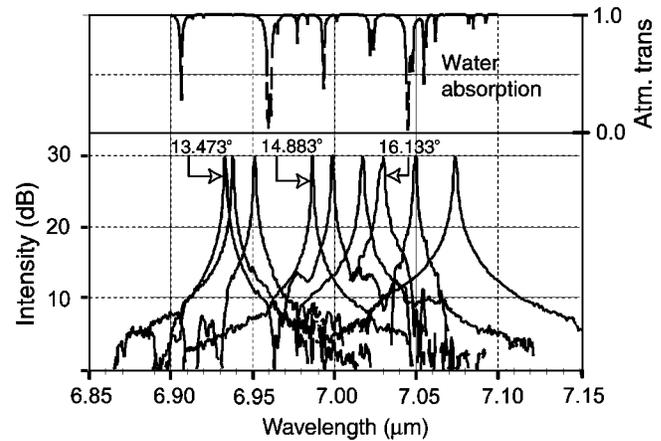
FIG. 2. Bottom: Laser wavelength tuning spectra obtained by tilting the mirror angle; a few angle values are shown. Top: Calculated atmospheric transmission for a distance comparable with the laser cavity roundtrip in air, showing strong water absorption. Wavelength tuning measurements were conducted within the water vapor windows.
