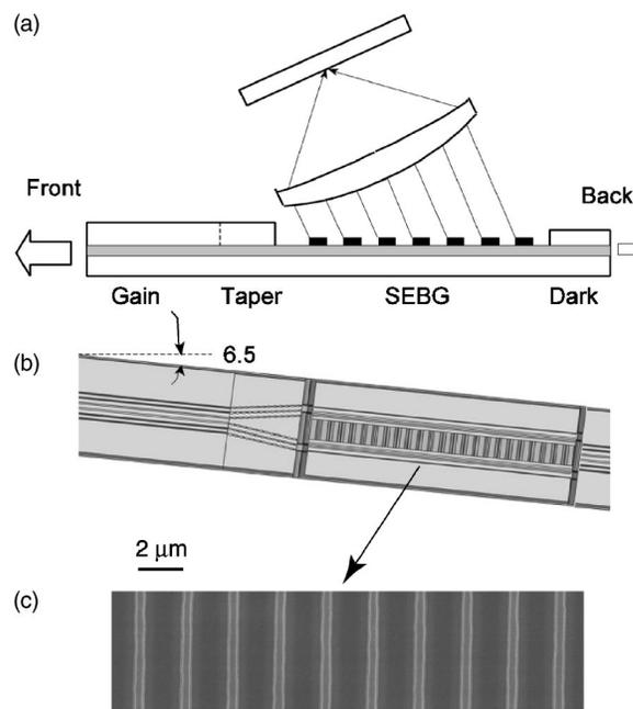
FIG. 1. (a) Schematic side view of the external cavity laser with off-band surface-emitting Bragg grating coupler; (b) Schematic top view of the device (the drawing is not to scale); (c) SEM image of the gratings.
