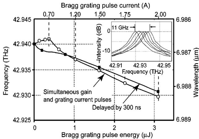
FIG. 3. Fine wavelength tuning behavior as a function of the surface-emitting Bragg grating injection current. The top axis shows the grating peak current, the bottom shows its pulse energy. Open circles: gain current  $I_g$  and grating current  $I_{BG}$  applied simultaneously. Filled square:  $I_g$  was delayed by 300 ns. Inset: examples of fine-tuning spectra.
